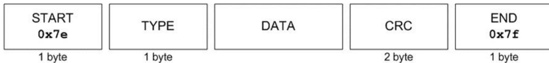
Figure 9.1: Structure of a data type
