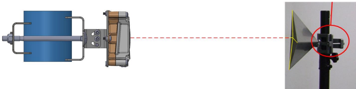
Figure 5.1: Mounting alignment of radar and reflector
