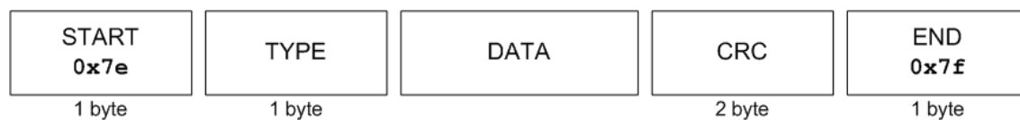
Figure 95: Structure of the data packet
