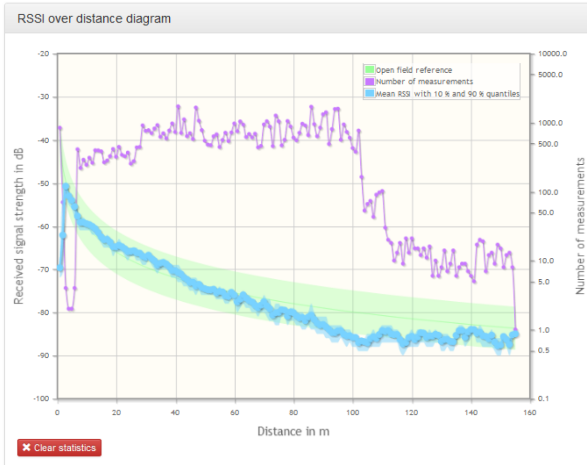
Figure 74: Diagnostics - RSSI over distance diagram
